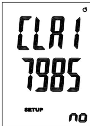
Fig. 5 Screen shows 17,985 readings left in memory.
