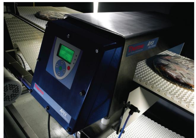
***When properly maintained and calibrated, an electronic metal detector, such as this one operating in a food plant, can reliably reject contaminated product for many years.***
